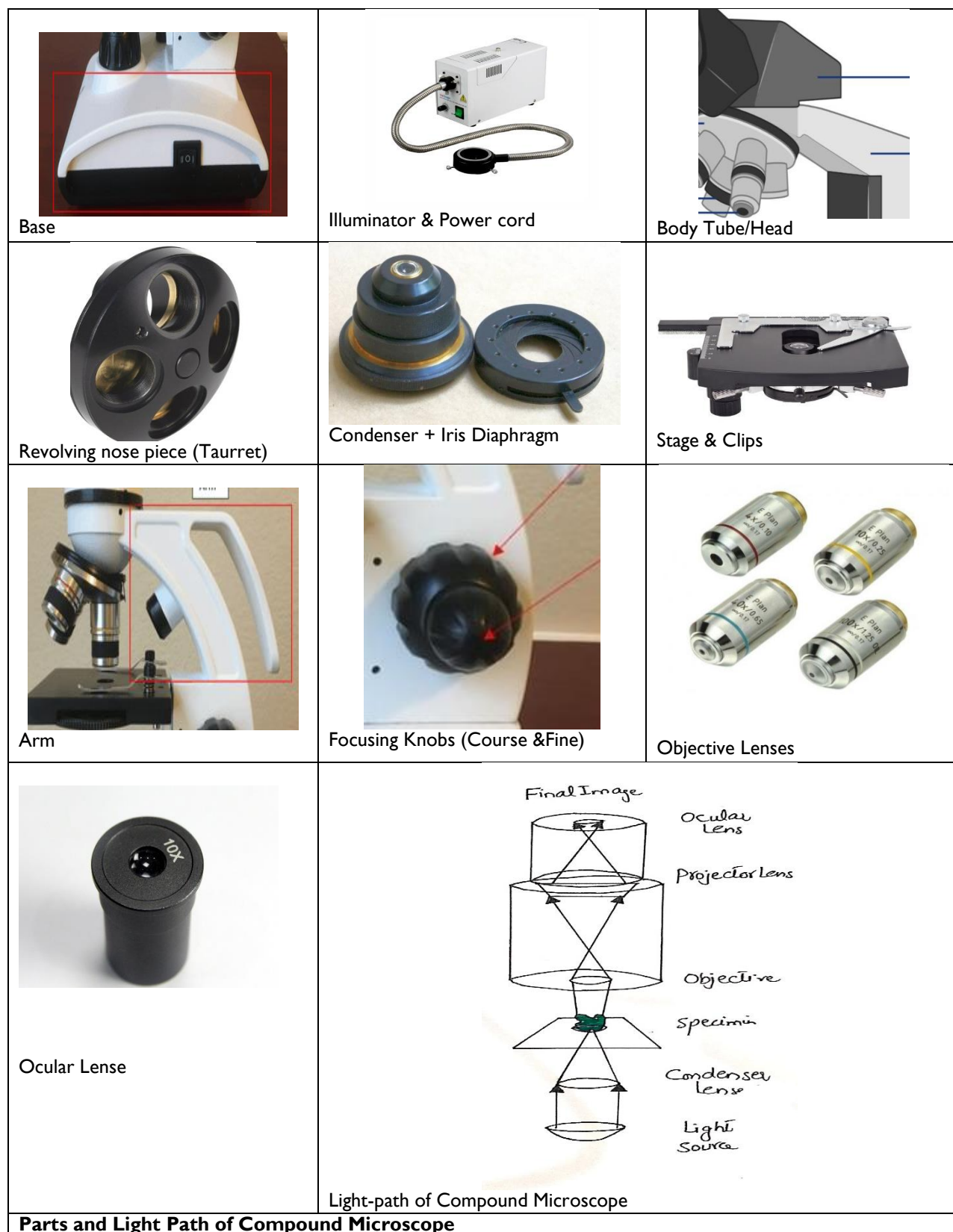
Figure 2: Parts and Ray Diagram of Binocular Bright-Field Compound Microscope
